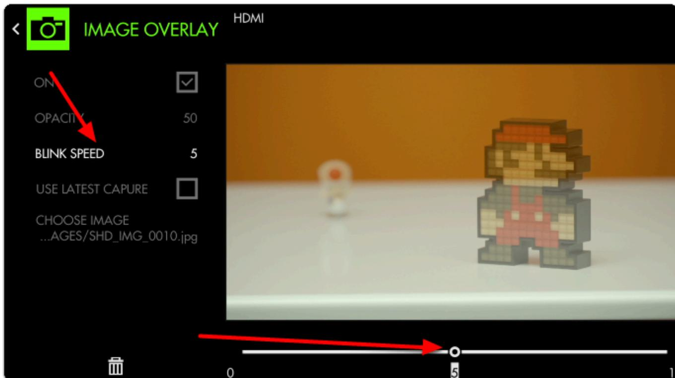
Increasing the **OPACITY** gives us a clearer distinction between the two images when blinking (if not set to blink, this will make the overlaid image completely opaque, covering the underlying feed)
