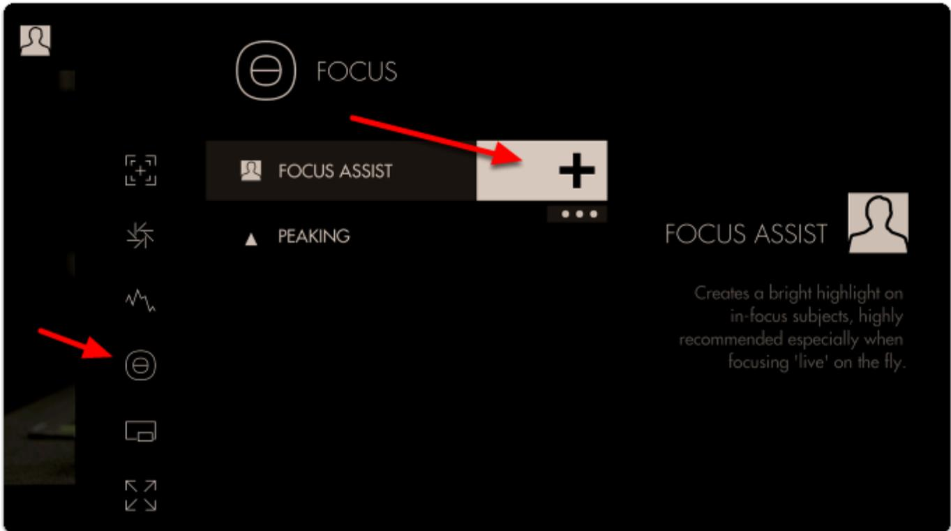
Once added you can **edit the settings** by **navigating right** or **tapping the right arrow** when 'Focus Assist' is highlighted.
