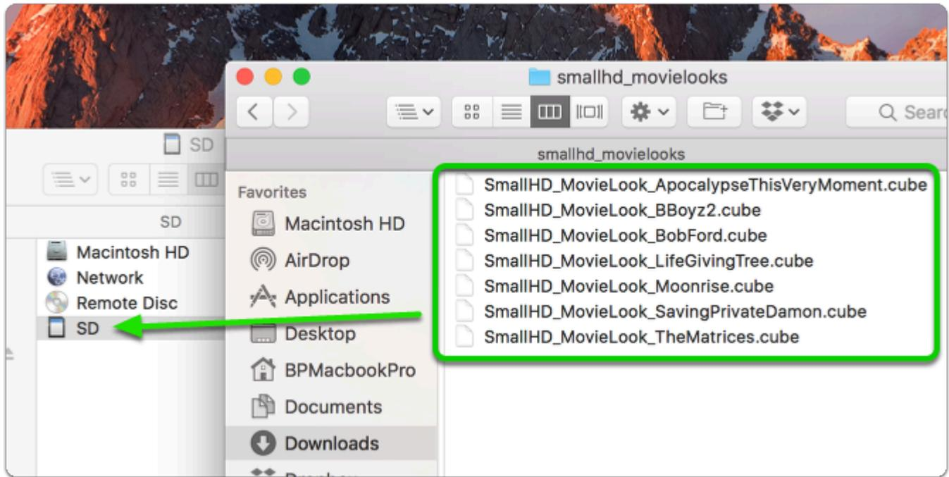
With the LUTs placed on the SD card, insert it into your monitor. From any page with a video feed, click the joystick or tap the screen to bring up 'Add New Tool' and navigate to Overlay > Look.
