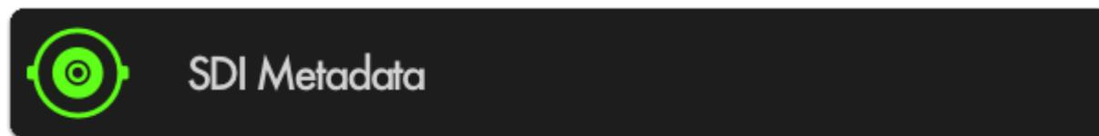
Displays a small information bar containing metadata information being sent over HDMI or SDI such as timecode and tally flags. Useful for ensuring the camera is recording without having to take your eyes off the monitor.
