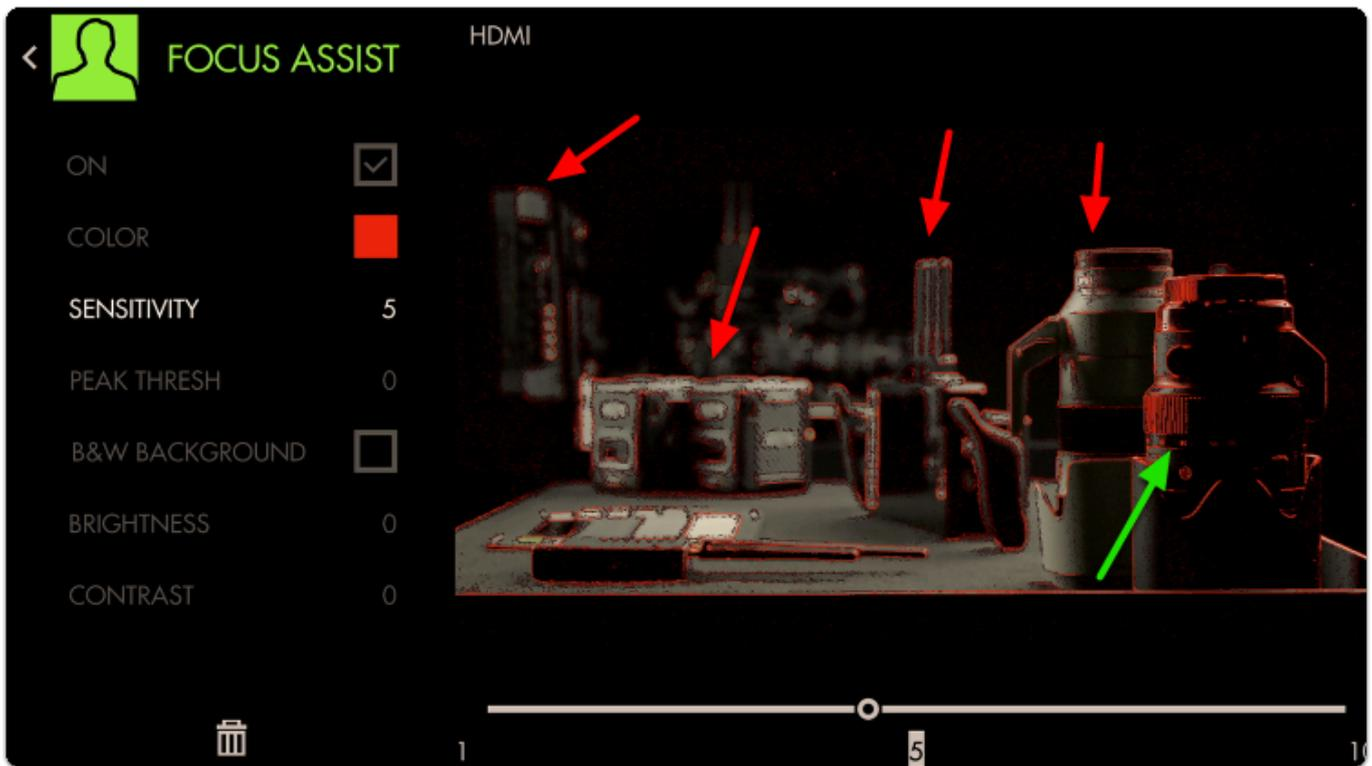
Notice how we are picking up many edges that are **not in focus** in addition to the areas that **are in focus**.
