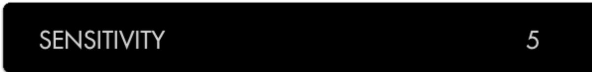
Sensitivity adjusts the intensity of Focus Assist - a low number causes a faint edge highlight, high numbers cause many more edges to be detected.
