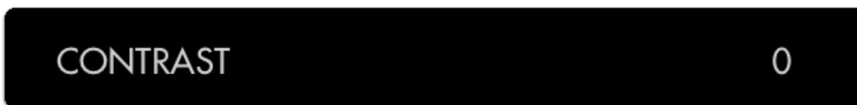
Adjust the brightness/contrast of the image to feed the Peaking filter with an adequate (ie not a flat log signal) source, translating into a clearer view of what is in focus.
