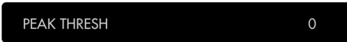
Peak Threshold is like a 'confidence' slider, the higher the Peak Threshold, the more confident Focus Assist needs to be about an area to paint it as 'in-focus'. Increase this setting to taste after increasing Sensitivity for best results.
