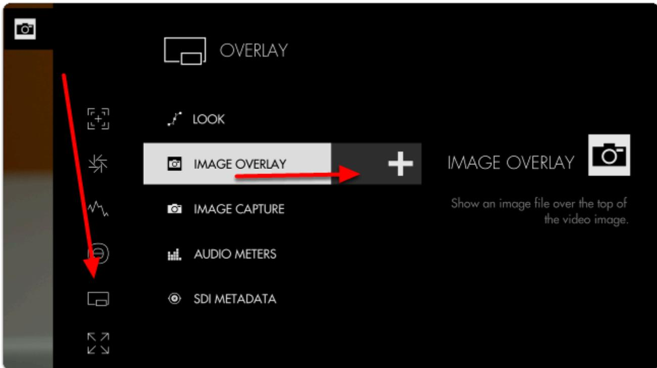
By default Image Overlay displays the **latest snapshot** taken with [Image Capture](#) at 50% opacity.
