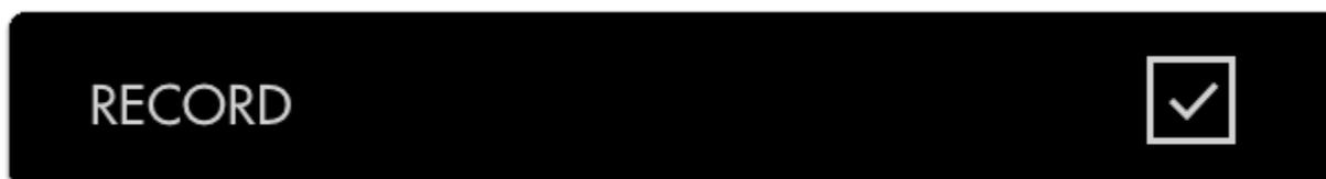
Enables display of the camera's record flag being sent over HDMI or SDI. This displays as a red rectangle around the edge of the monitor.
