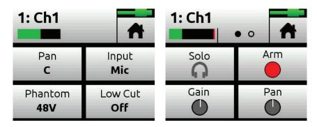
In Advanced mode, additional settings are available via a second channel page accessed by tapping the Dots icon.
